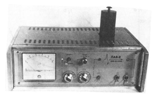
Fig. 3. Home-made luminescent analyser of moisture.
