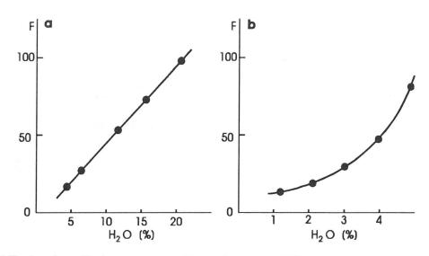
Fig. 5. The dependence of luminescent parameters (F) on moisture content (%  $H_2O$ ) for dried milk (a), and grain (b). T = 23 °C.
