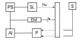
**Fig. 2.** Block-scheme of luminescent analyser. PS-power supply, SL-source of light, EM-electromechanical modulator, P- photomultiplier, AI - analog indicator, S-sample.
